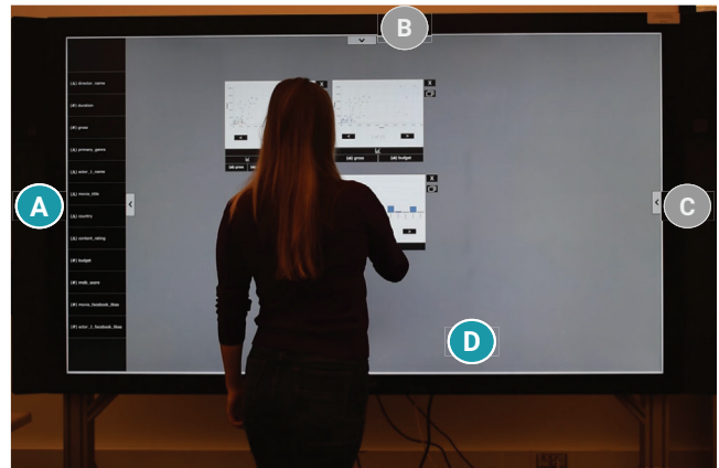
Figure 1: A user exploring the movies dataset on VisWall running on an 84" Microsoft Surface Hub. (A,B,C) Attribute panels and (D) Visualization Canvas. In this case, only one of the attribute panels (A) is open.
