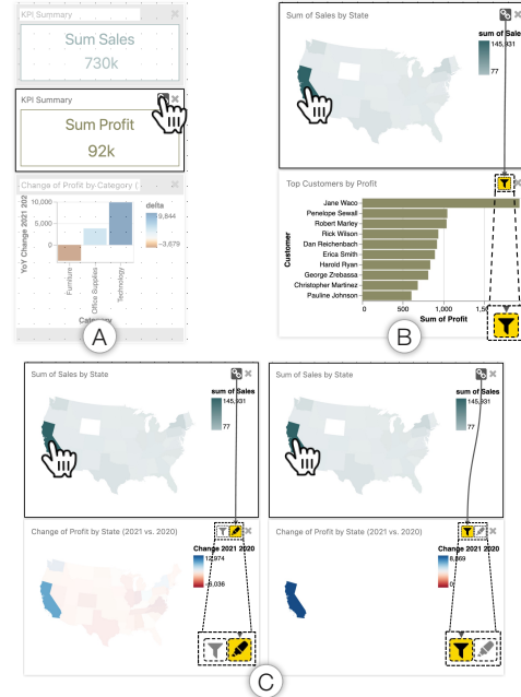
Fig. 6. MEDLEY's dashboard interaction scenarios based on Figure 1C. (A) An example where a view cannot be used to interactively update other views in the dashboard. (B) An example where a source view can only be used to filter items in the target view. (C) An example where both highlight and filter interactions are possible between two views.
